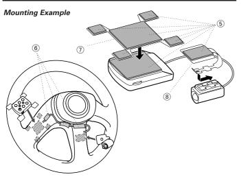
Attach the operation section and the light emitting section of the Steering Remote Control as shown above. Be sure to attach them to positions that can ensure proper
